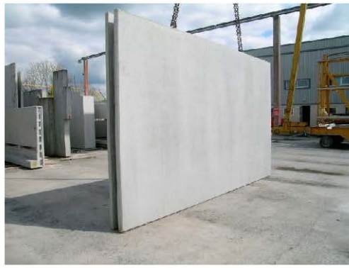
Precast double walls
