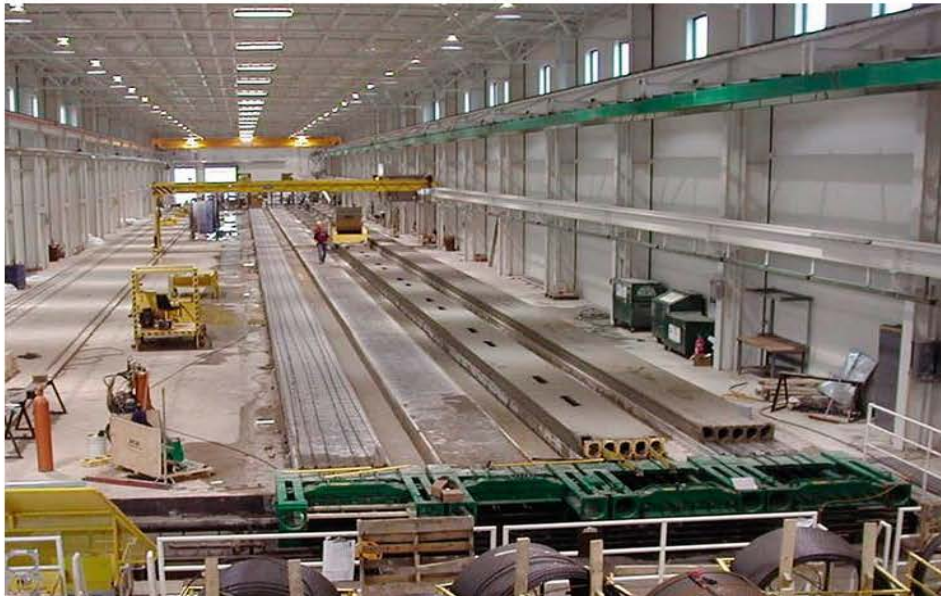
Long line Hollow Core Slabs production
